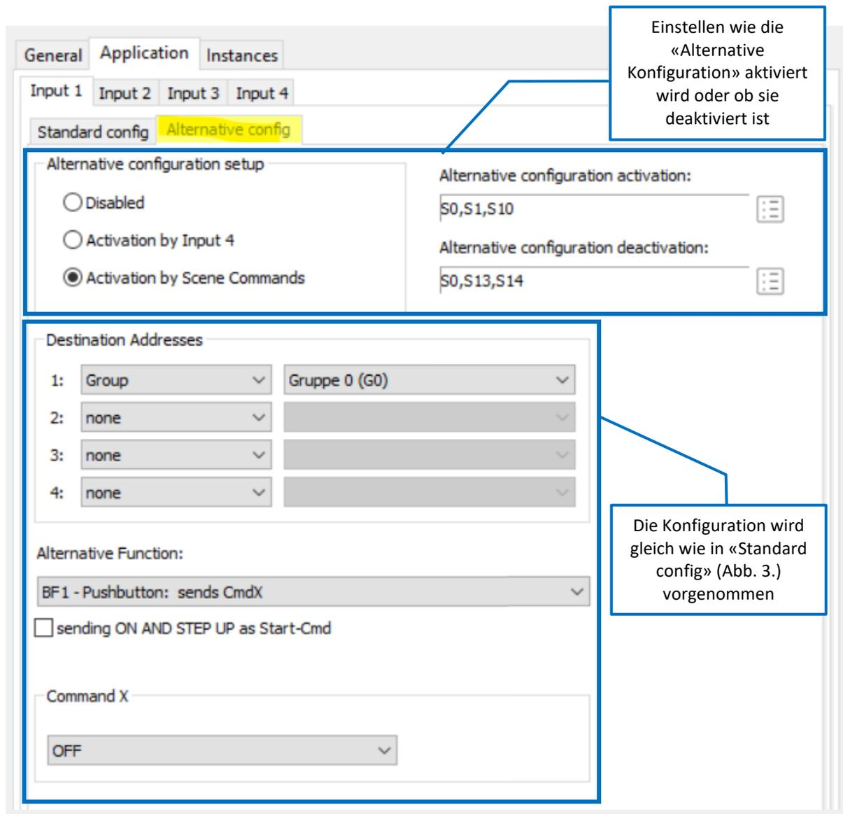
Abb. 8 Alternative Konfiguration
