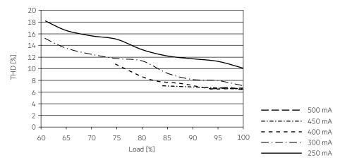
100 % load corresponds to the max. output power (full load) according to the table on page 2.
